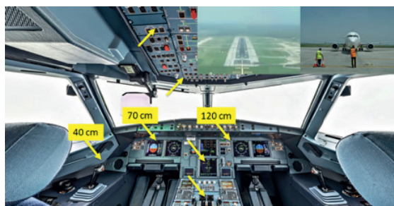
Figure. Pilots work in a complex visual environment requiring clear vision at a variety of distances inside and outside of the cockpit. Arrows indicate controls and displays located at near and various intermediate visual distances.
