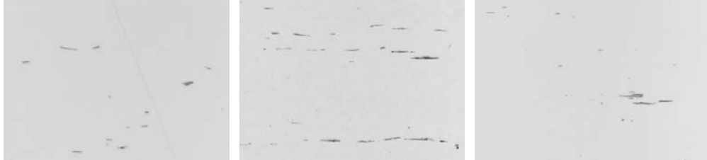
Sulphide inclusions in steel With kind permission of SKF GmbH, Schweinfurt, Germany
