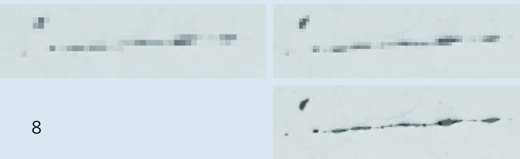
Improving the display of inclusions by changing the resolution
