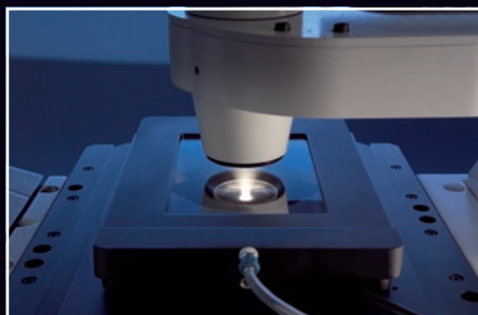
Fig. 1: Optimum incubation conditions, more space: incubator PM S1 for Petri dishes and multiwell plates.
