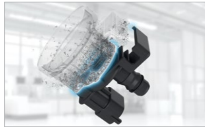
Porosity analysis of a media carrying plastic part
