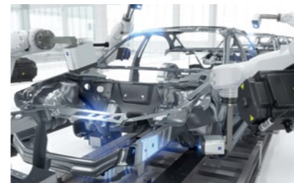
Optical inline inspection of the Battery Tray
