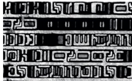
Passive Voltage Contrast Image of an Integrated Circuit (IC) Using Electron Microscope
