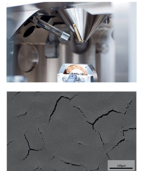
Electron microscope image of an electrode coating including crack network
