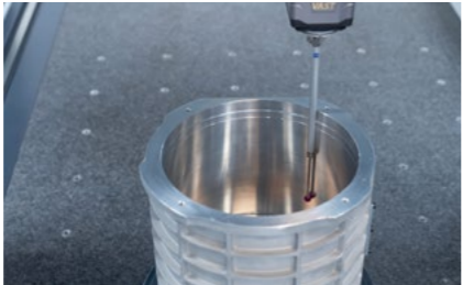
Measurement of Housing with ZEISS Tactile Scanning Technology
