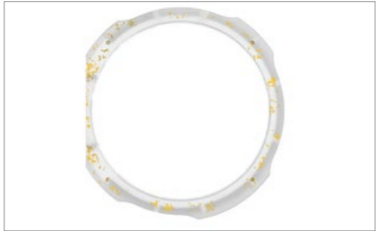
3D X-ray Scanning Data and Evaluation of Casting Defects in Cross Section
