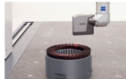
Laser Scanning of the Stator – Handheld or Automatically on ZEISS CMM
